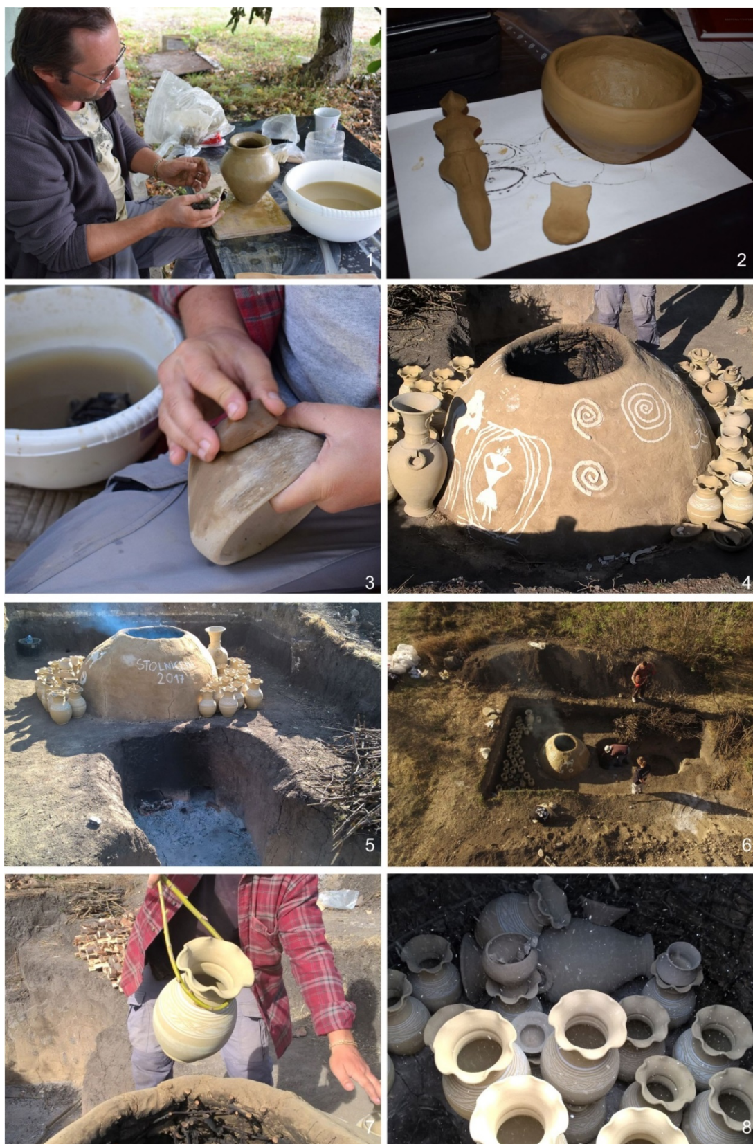
Pl. IV. 1-3. Making pottery to be fired in the kiln; 4-5. The unfired pottery, ready to be loaded in the kiln; 6. The kiln place, view from above; 7-8. Loading the kiln (photos by the authors).
